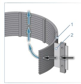
The filter systems are designed for extremely stable and robust applications. They consist essentially of the following components: Two-piece filter housing, wedge wire element (1), holding plate with scraper (2) gear drive. The filtration is through the wedge wire element from outside to inside, wherein the solids accumulate on the outside of the wedge wire element.
